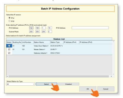
Typically, stations deployed across a managed network cannot be found by Support Tool unless the network is configured to allow this broadcast search. In this case, it may be easier to move the stations to a switch local to the programming PC than it would be to configure the network to allow a network-wide broadcast.
