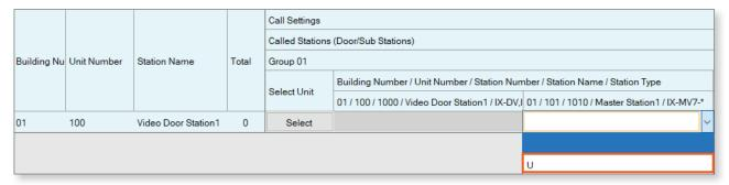
The door stations can only be set to ring one unit of mobile apps per group. To select the desired unit's mobile apps, scroll to the right and click **Select**. Place a check mark next to the desired mobile app unit and click **OK**.
