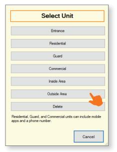
Once all units have been added, enter a <u>Unit Name</u> for each. For each station to be added to a unit, click <u>Select</u> next to the appropriate station in that unit and choose a station type from the list. Use the drop-down menu to select how many mobile apps are permitted for each unit, if needed.
