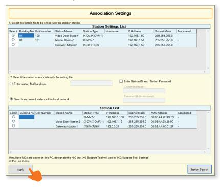
Typically, stations deployed across a managed network cannot be found by Support Tool unless the network is configured to allow this broadcast search. In this case, it may be easier to move the stations to a switch local to the programming PC than it would be to configure the network to allow a network-wide broadcast.
