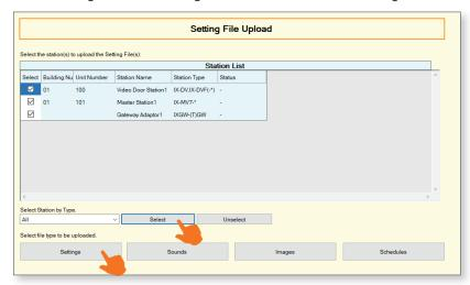
If any stations fail, they may still be booting up from the Association Settings step. It is also important to ensure that the programming PC is in the same subnet range as the stations. For example, if the stations are set to 192.168.1.xx, the PC should also be set to this.
