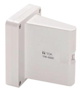
The wireless antenna YW-4500 has been designed for UHF band wireless system. Cable loss can be compensated for by a built-in RF signal booster. The YW-4500 in a dipole antenna designed to be installed indoors. Use the coaxial cable with 75  $\Omega$  impedance.
